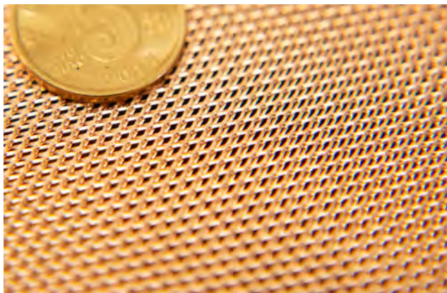
The copper and aluminum expanded metal foils is widely used on the composite blade material manufacturing for lightning striking protection, preventing the damage from lightning striking and extending the blade service life.
